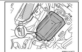
5. Disconnect harness connector and then remove IPDM E/R ① from IPDM E/R cover B ②.
