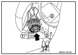
Disengage push-button ignition switch fixing pawl and then remove push-button ignition switch ① from NATS antenna amp.
